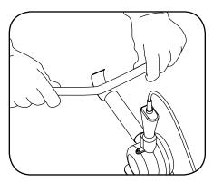
**Part 2:** The workable forming time is about 2–3 minutes. The light guide must remain in the desired position until completely cooled. See the chart above for minimum bend radius auidelines.
