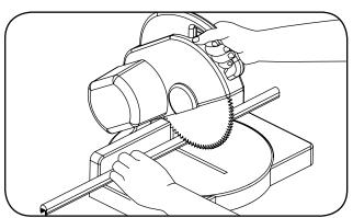
3 Cut the light guide to the required length using a hacksaw, chop saw (cross cut or veneer blade only), band saw, or other appropriate plastic cutting tool.
