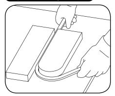
Preheat the heating equipment to 300°F (149°C). Heat light guides approximately 6-15 minutes until soft and pliable. Bend the light guide over a printed pattern, routed template, or use free-forming. A clean flat insulated surface (wood or laminated countertop) will help to prevent twisting or bowing. See the chart above for minimum bend radius guidelines.
