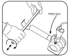
**Part 1:** Move the section back and forth while rotating about the diameter until it is soft and pliable. Gently bend to the desired angle.
