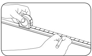
2 Mark the light guide at the required length, adding 0.5 in. (13mm) for every 16 in. (406mm) to account for shrinkage during the forming process.
