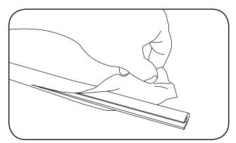
• Remove the protective film from the light guide.
