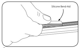
4 Fill the entire light guide channel with the GEXNBA Silicone Bend-Aid(s) and press into place. Bend-Aid must be installed prior to heating and forming.
