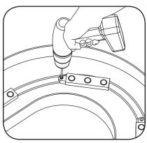
Use rivets, screws, or silicone to secure at least every fifth LED module within the channel letter. Use #6 (M3) or #8 (M4) pan headed metal screws, 1/8-inch (3.2 mm) rivets, or silicone.
