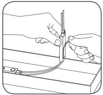
Remove tape backing and stick LED modules into place.
