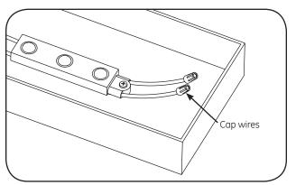
Must cap all exposed wires with appropriate wire connectors.
