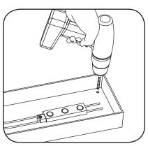
**5** Drill a 1/4" (6.4 mm) hole near the LED strip and grommet the hole for supply wire access.
