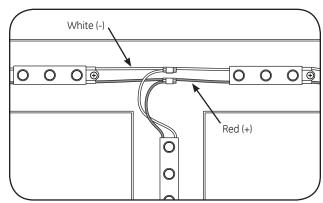
Connect LED strips using in-line (IDC) connectors or twist-on wire connectors.
