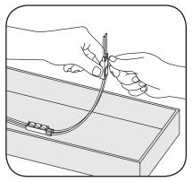
Remove tape backing and stick LED modules into place. Continue until you have reached the end of the strip.
