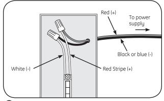
Connect the red stripe wire (+) of the LED strip to 4 the red wire (+) of the power supply. Connect the white wire (-) of the LED strip to the black or blue wire (-) of the power supply.
