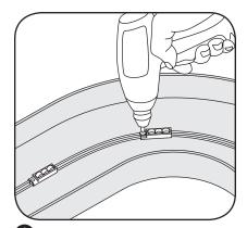
Use rivets, screws, or silicone to secure at least every fifth LED module within the channel letter. Use #6 (M3) or #8 (M4) pan headed metal screws, 1/8inch (3.2 mm) rivets, or silicone.
