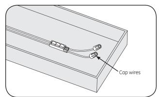
Must cap all exposed wires with appropriate wire connectors or electrical grade silicone or equivalent.
