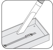
6 Clean and remove all debris from the inside of the channel letter. Replace sign face.
