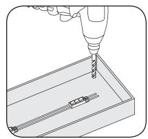
5 Drill a 1/4-inch (6.4 mm) hole near the LED strip and grommet the hole for supply wire access.
