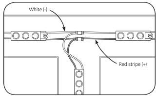
1 Connect LED strips using in-line (IDC) connectors or twist-on wire connectors.
