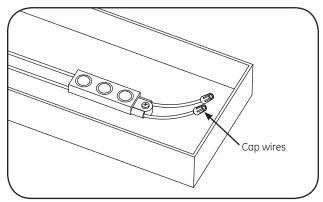
2 Must cap all exposed wires with appropriate wire connectors.
