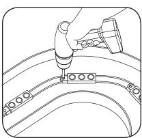
4 Use rivets, screws, or silicone to secure at least every fifth LED module within the channel letter. Use #6 (M3) or #8 (M4) pan headed metal screws, 1/8-inch (3.2 mm) rivets, or silicone.
