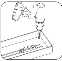
5 Drill a 1/4-inch (6.4 mm) hole near the LED strip and grommet the hole for supply wire access.
