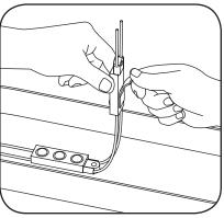
3 Remove tape backing and stick LED modules into place. Continue until you have reached the end of the strip.
