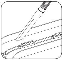
6 Clean & remove all debris from the inside of the channel letter. Replace sign face.
