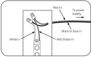
4 Connect the red stripe wire (+) of the LED strip to the red wire (+) of the power supply. Connect the white wire (-) of the LED strip to the black or blue wire (-) of the power supply.
