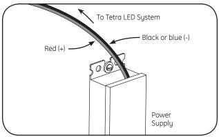
3 Run a wire from the Power Supply to each channel letter and connect to the first LED module on the strip.
