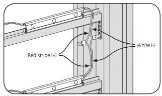
1 Connect modules using twist-on wire connectors or in-line (IDC) connectors. Join white wires together and red striped wires together.
