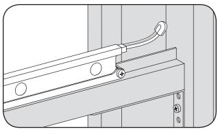
Cap all exposed wires with appropriate end caps or apply electric grade (non-corrosive) silicone for additional weather protection.
