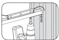
Secure the Mounting Rail to the inside of the box sign using a Tetra<sup>®</sup> Mounting Rail Bracket or other suitable mounting means. Ensure the #6 (M3) screw does not exceed 3/4 inches (19 mm) in length.
