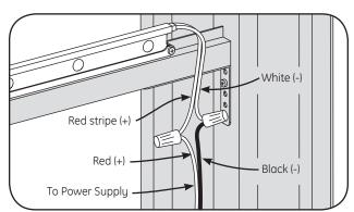
Connect the red stripe wire (+) of the LED system to the red wire (+) of the power supply. Connect the white wire (-) of the LED system to the black wire (-) of the power supply.
