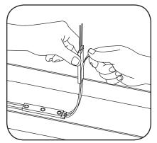
Remove tape backing and stick LED modules into place. Continue until you have reached the end of the strip.
