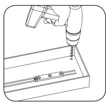
Drill a 1/4" (6.4 mm) hole near the LED strip and grommet the hole for supply wire access.
