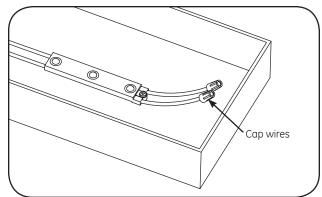
Must cap all exposed wires with appropriate wire connectors.
