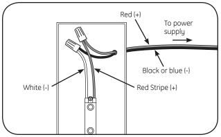
Connect the red stripe wire (+) of the LED strip to the red wire (+) of the power supply. Connect the white wire (-) of the LED strip to the black or blue wire (-) of the power supply.
