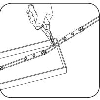
Measure and cut Tetra® LED strip to the appropriate length for each letter. Cuts can be made between any of the modules.
