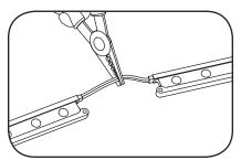
2 Determine how many modules are required for one row and cut wire.
