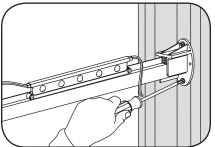
Secure the Mounting Rail to the inside of the box sign using a Tetra® Mounting Rail Clip or other suitable mounting means. Ensure the #6 (M3) screw does not exceed 3/4 inches (19 mm) in length.
