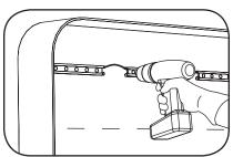
Secure with at least one screw per module with #6 or #8 (M3 or M4) screws or 1/8-inch rivets (3.175 mm), silicone or equivalent.
