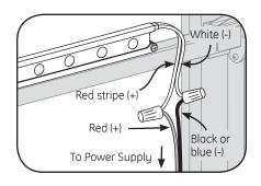
Connect the red stripe wire (+) of the LED system to the red wire (+) of the power supply. Connect the white wire (-) of the LED system to the black or blue wire (-) of the power supply.
