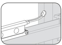
2 Cap all exposed wires with appropriate end caps or apply electric grade (non-corrosive) silicone for additional weather protection.
