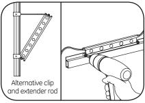
Arrange modules evenly spaced apart. Place the Tetra® modules on the Mounting Rail and secure into lip with a self-tapping #6 (M3) screw or 1/8-inch (3.175 mm) rivet. Or mount using the alternative clip and extender rod configuration.
