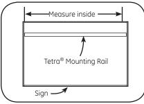
1 Measure and cut Tetra® Mounting Rail or other suitable mounting means to appropriate length to fit into sign.
