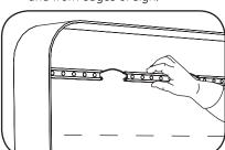
Position string of modules ene to end along guidelines inside of sign. Evenly space modules by arranging approximately one module per 12 inches (305mm).
