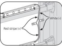
Connect modules using twist-on wire connectors or in-line (IDC) connectors. Join white wires together and red striped wires together.
